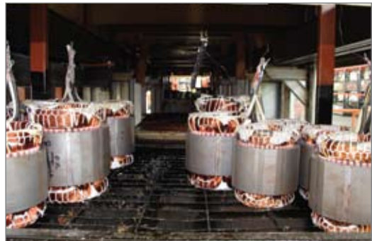
Automatic Impregnation Plant
