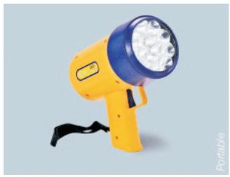
Consist of multi LED lamp, automatically switches – **ON**, on mains power failure & provides illumination on battery source for specified duration, after which the battery gets automatically cut-off, to facilitate quick recharge on the resumption of mains supply. Once the battery is fully charged, it automatically slides into trickle charge to constantly retain the charge and be ready for immediate use.
